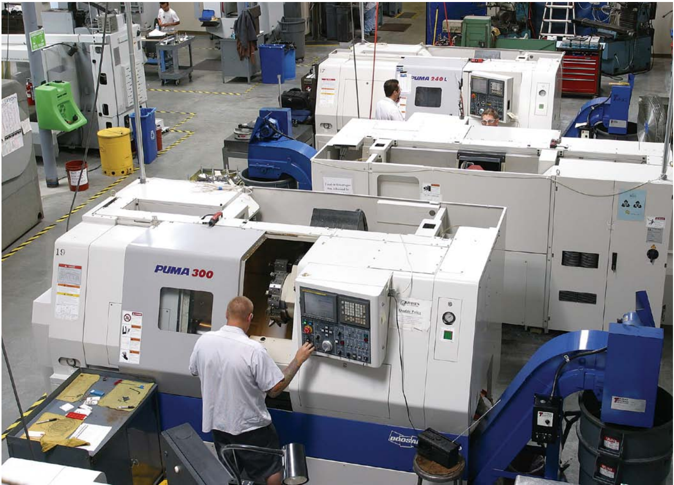
Overview of the Jerames shop floor showing three of the company's four Doosan Puma CNC turning centers. Jerames operates a Puma 240 CNC, two Puma 300s and one Puma 300 with live tooling. In addition, the equipment lineup includes a number of 5- 4- and 3-axis Haas machining centers. Predator DNC is used to communicate with the equipment from a central server. The company currently employs 26 people in a modern new facility.
